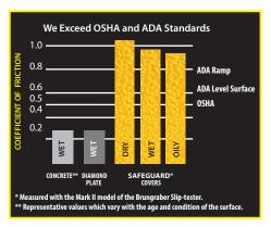
'Safeguard incorporates Fused Alumina as the aggregate in it's Anti-Slip surface. This abrasive is characterized by a sharp edged particle shape and measures (9.0) on the Moh's Hardness Scale for abrasives. This ranks just below Diamond (10). Comparatively, most tapes and paints incorporate quartz or silica, which are synonyms for sand, as the aggregate. These rank only in the 6-7 range on the scale.
