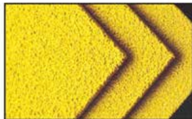
A sample of available grades, left to right: Offshore/Heavy Duty-Extra Coarse, Industrial-Coarse, and Commercial-Fine ⓘ
